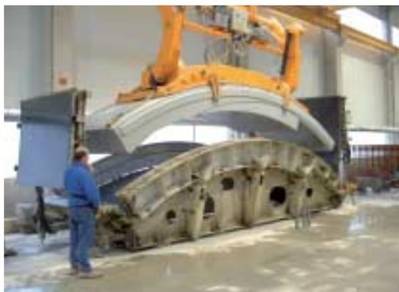
Fig. 3 Production of tubings.
